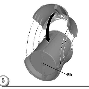
• Fit the remaining outer column piece onto the inner column. *Hint:* Line up the groove in the outer column piece with the rib on the inner column.
